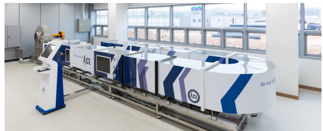
Figure 3. ASHRAE 52.2 Test Wind Duct.
