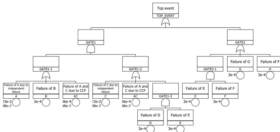
Fig. 3. The configuration of the fault tree used in example studies.
