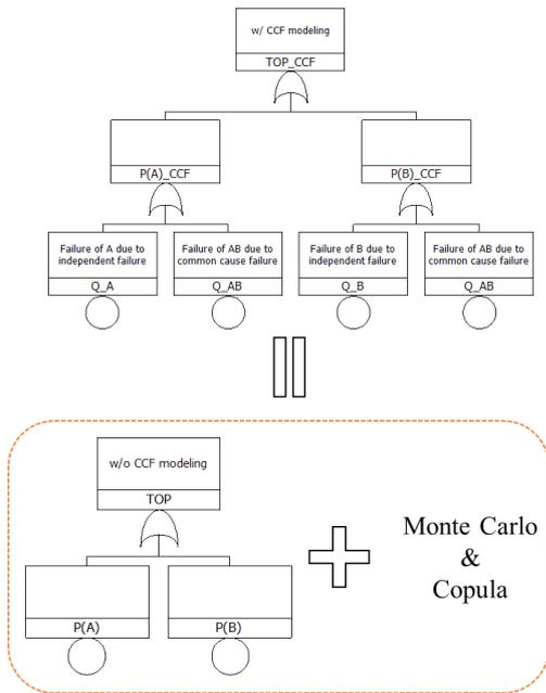
Fig.2. The concept of the estimation of the dependent failure probability without a CCF modelling using a copula and MC simulation.
