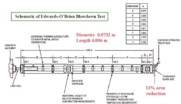
Figure 3 Schematic diagram of Edward Pipe
