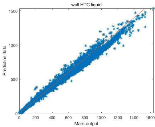
Figure 10 Wall heat transfer coefficient film regime
