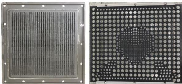
Fig. 1. Test section of CBSG heat exchanger unit and the perforated plate
