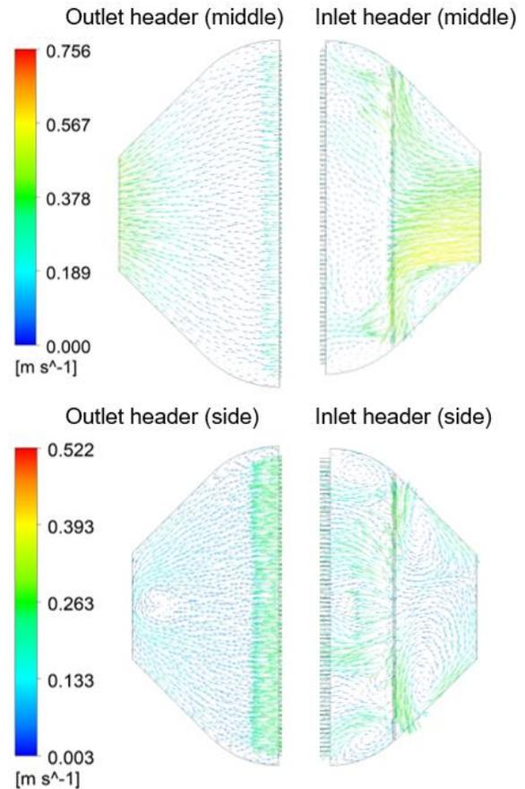
Fig. 5. The velocity field in the vertical middle and side planes in the inlet and outlet headers for proposed design with a perforated plate.
