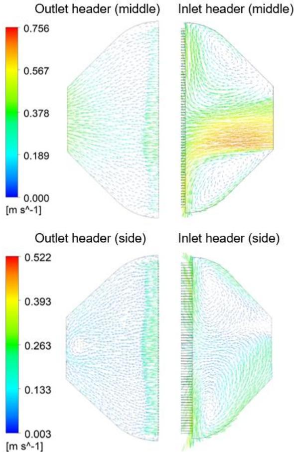
Fig. 4. The velocity field in the vertical middle and side planes in the inlet and outlet headers for original design
