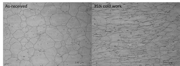
Fig. 2. Microstructure of as-received and 35% cold work materials
