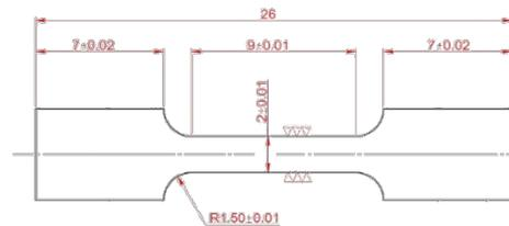
Fig. 1. Geometry and dimension of miniature tensile specimen for irradiated materials
