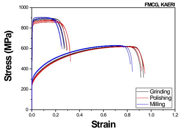
Fig. 4. Stress-strain curves of as-received material and 35% cold work material with different surface finishing method
