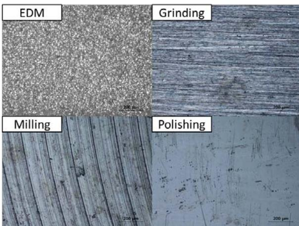
Fig. 3. Surface conditions of miniature tensile specimens with different surface processing method
