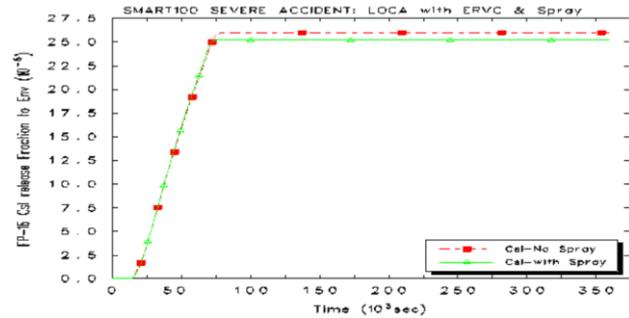
Fig. 2.3.1 CsI release fraction to environment
