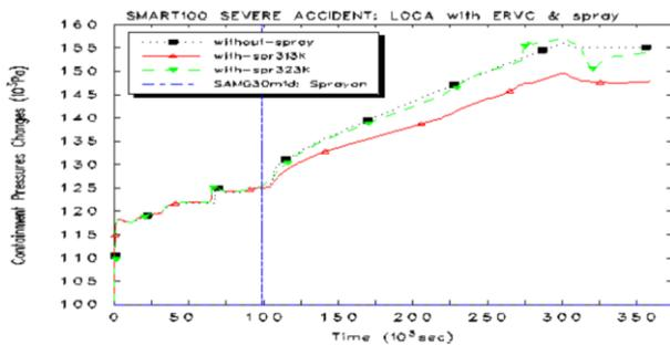
Fig. 2.2.1 Pressure of the containment (UCA)
