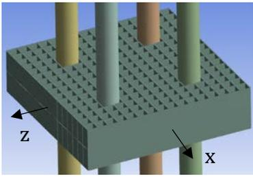
Fig 6. Beam model of spacer grid
