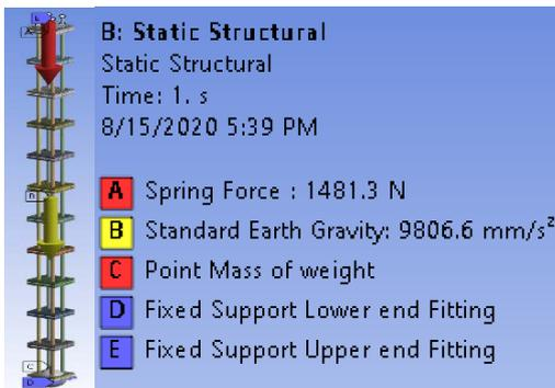
Fig 7. Boundary condition of nuclear fuel assembly
