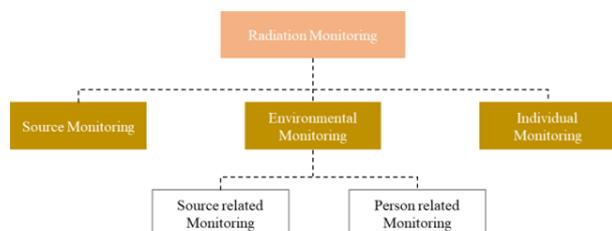
Fig. 1. Three types of radiation monitoring for the public[1]
