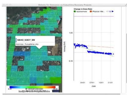
Fig. 9. Measurements by KURAMA- II mounted on local circular buses in Fukushima Prefecture
