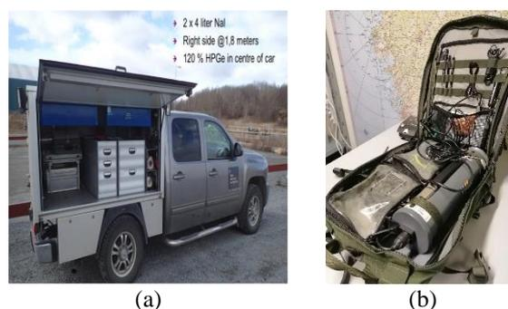
Fig. 4. Mobile radiation measuring systems in Sweden (a) vehicle-type gamma spectroscopy, (b) backpack-type monitoring system
