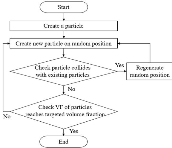
Fig. 2. Generation algorithm for random position of the  $Y_2O_3$  particles
