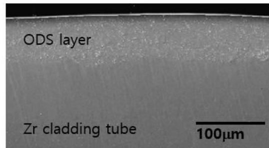
Fig. 1. Cross-sectional SEM images of the ODS Zircaloy-4 [3]
