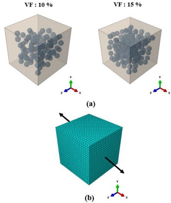
Fig. 3. (a) 3D RVE model of the ODS layer with different VF of the  $Y_2O_3$  particles and (b) loading for the elastic simulation
