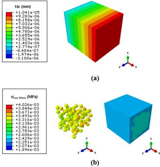
Fig. 4. Simulation results of (a) displacement along the X direction and (b) von Mises stress distribution of the  $Y_2O_3$  particles and Zircaloy-4 substrate for the 3D RVE model with VF of 10 %.
