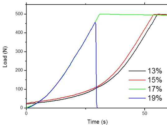
Fig. 3. Load as a function of time obtained tensile test for cladding samples with different ECR.
