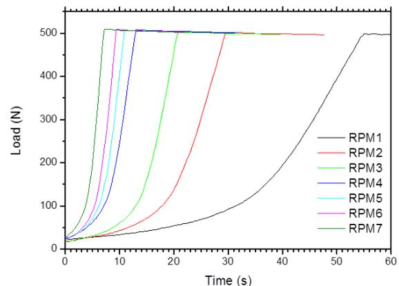
Fig. 1. Load obtained tensile test performed at room temperature with different RPM of motor.
