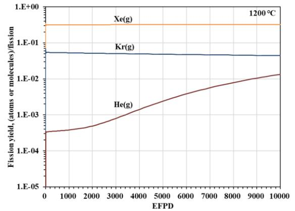
Fig. 2. Variation of the fission yields of gases produced in a TRISO.
