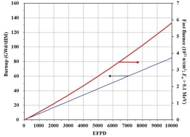
Fig. 1. Variation of fuel burnup and fast fluence.
