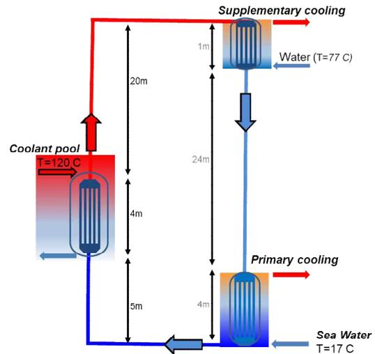
Fig. 3 Modeling design of WCPDHRS
