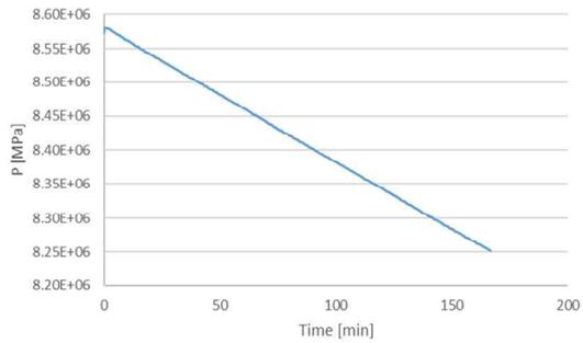
Fig. 7 Calculation results of containment pressure of UCPDHRs
