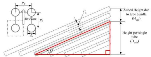
Fig. 5 Reference heat exchanger design layout
