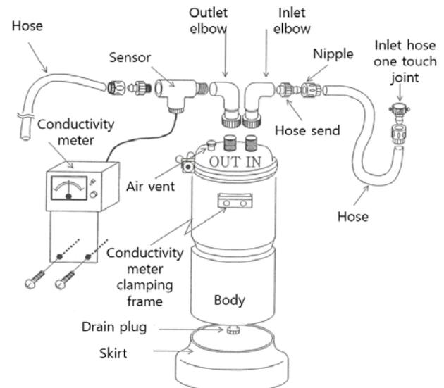
Fig. 2. An assembly diagram of the C-5P type ion exchanger
