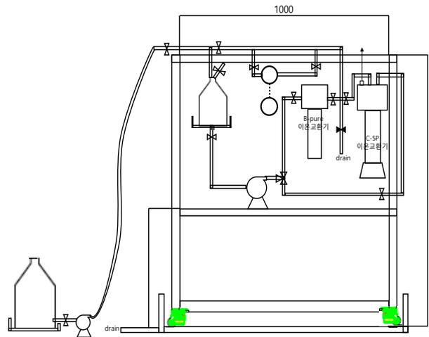
Fig. 1. Schematic diagram of ion exchange resin saturation loop developed in this work
