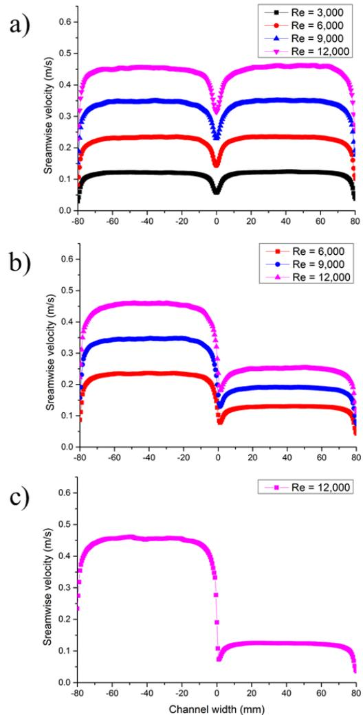
Fig. 3. Streamwise mean velocity profiles at the plane 0 of inlet with different inlet conditions: a) Uniform (5:5) b) Non-uniform (6.5:3.5) c) Non-uniform (8:2)
