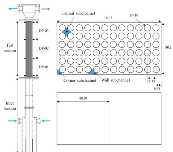
Fig. 1 Schematic diagram of PRIUS-II and cross sectional views of test section (Rod bundle) and inlet section.
