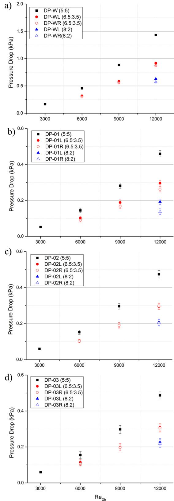
Fig. 4. Pressure drop measured at test section: a) Whole range of test section b) DP-01 c) DP-02 d) DP-03
