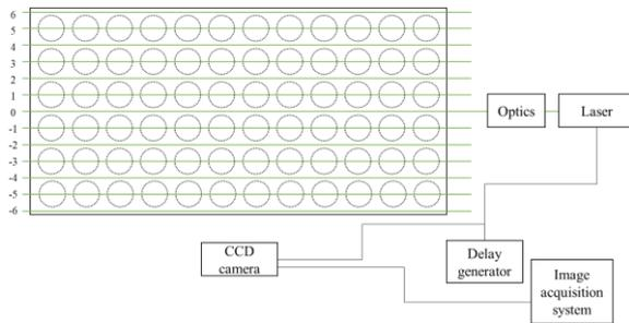
Fig. 2 Schematic of PIV measurement system.
