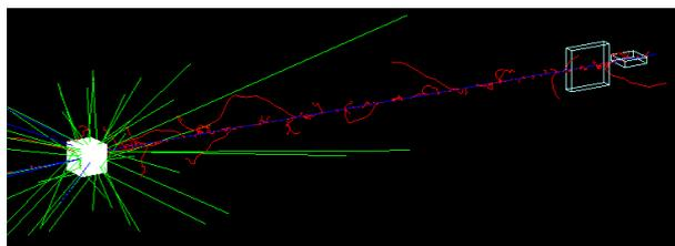
Fig. 1. Graphical representation of TOPAS model of active beam scanning system. Green lines mean gammas, red lines mean electrons, blue lines mean carbon ions.
