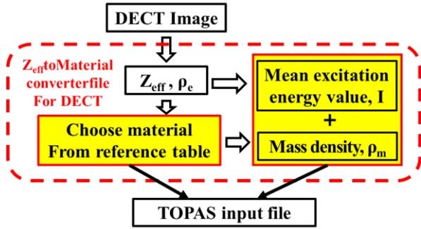
Fig. 2. Schematic diagram of the process of extracting the information necessary for dose calculation from the DECT image and making it an input file of TOPAS
