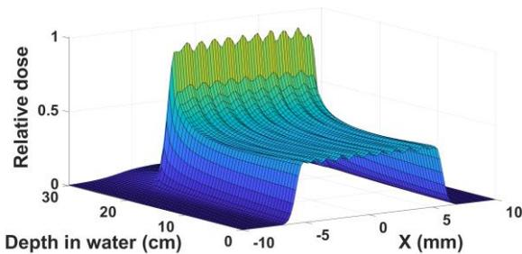
Fig. 3. IDD curve of 350 MeV/u monoenergetic carbon ion beam in water phantom.
