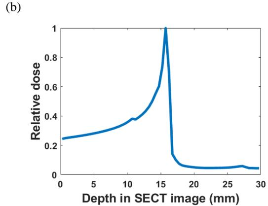
Fig. 4. (a) Raw SECT image (down, right) and SECT image imported to TOPAS (down, left). (b) IDD curve of 80 MeV/u monoenergetic carbon ion beam after beam is scanned on SECT images.
