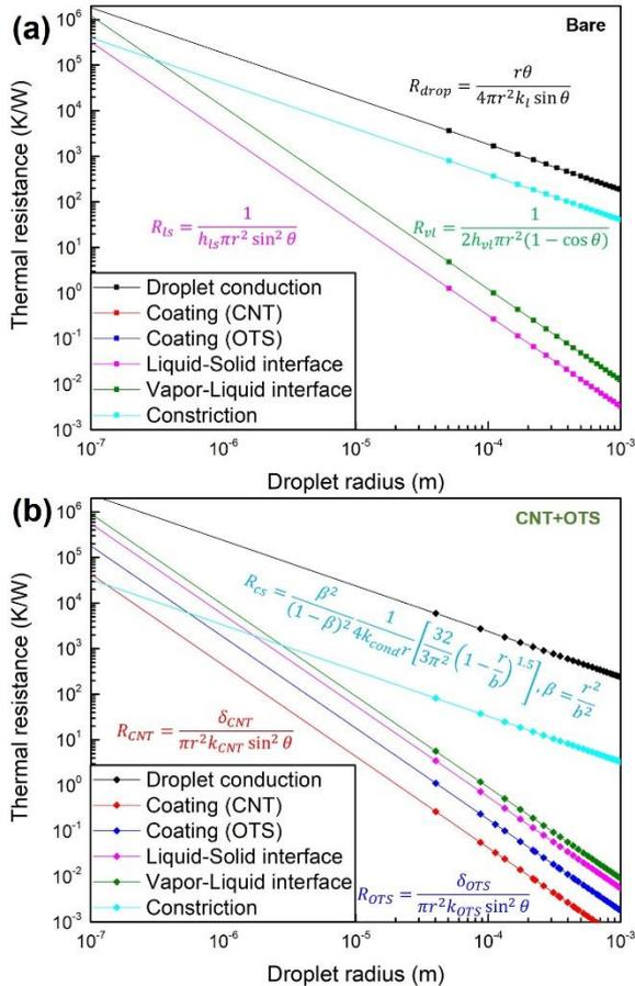
Fig. 7. Thermal resistance of bare and CNT+OTS surfaces on the dropwise condensation [3,5,7]
