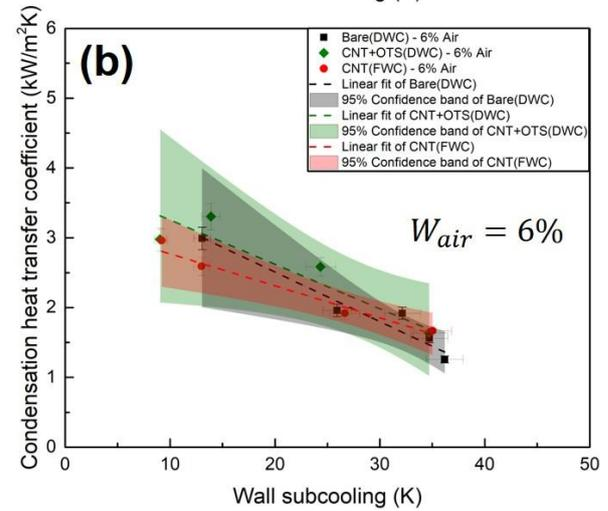
Fig. 8. The condensation heat transfer coefficient surfaces on the steam-air mixture condition (3, 6%).
