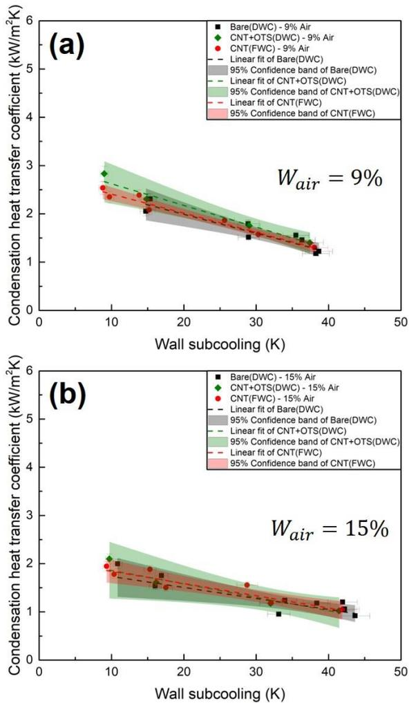
Fig. 9. The condensation heat transfer coefficient surfaces on the steam-air mixture condition (9, 15%).
