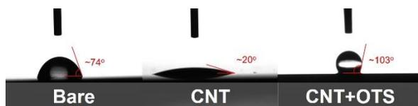
Fig. 3. Static contact angle of the bare, CNT, and CNT+OTS surfaces
