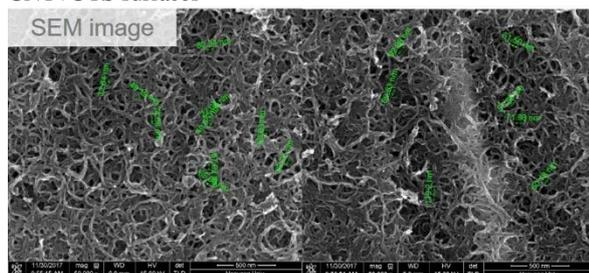
Fig. 4. SEM images of CNT layers
