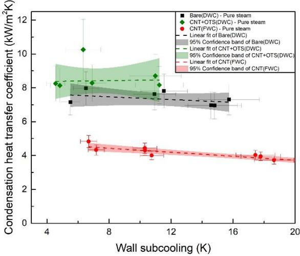
Fig. 6. The condensation heat transfer coefficient of bare and modified surfaces on pure steam condition.
