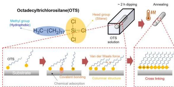
Fig. 2. A schematic for fabrication of OTS monolayer coatings on the substrates
