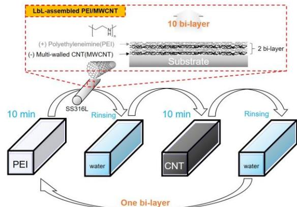
Fig. 1. A schematic illustrating fabrication of LbL-assembled PEI/MWCNT coatings on the substrates
