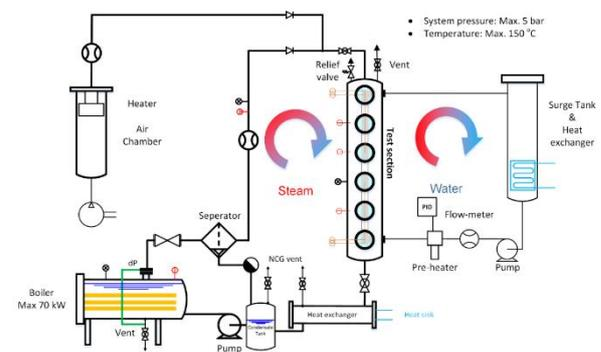
Fig. 5. A schematic of condensation heat transfer experimental system
