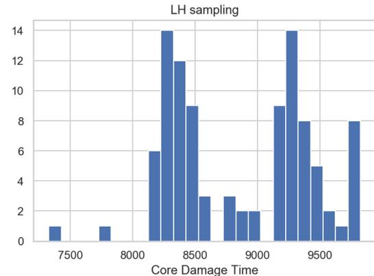
Fig. 6. Core Damage Time Distribution by LHS
