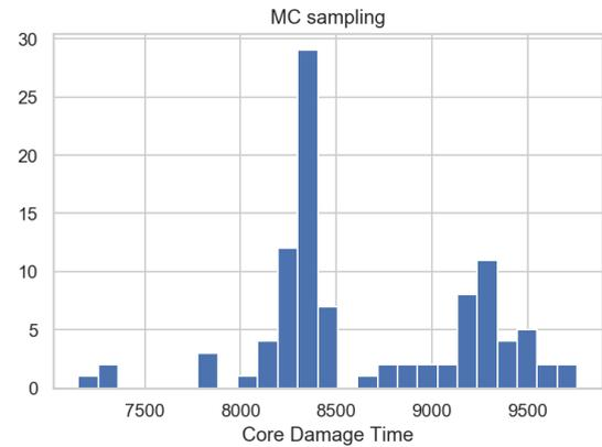
Fig. 5. Core Damage Time Distribution by MCS
