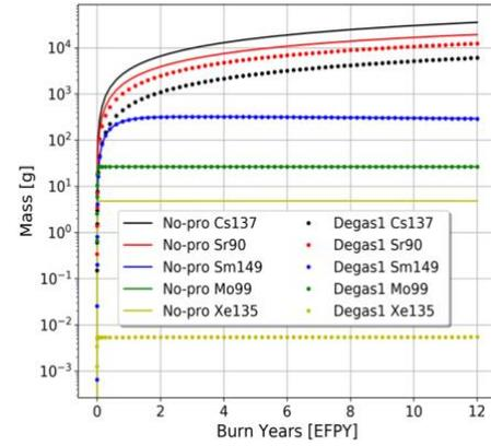
Figure 5. The mass of FPs in fuel salt of no-pro and Degas1.
