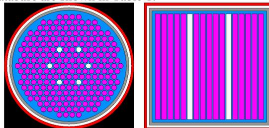
Figure 1. The layout of the CMSR reactor in Serpent 2 code.
