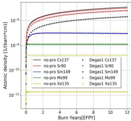
Figure 4. The atomic density of FPs in fuel salt of no-pro and Degas1.
