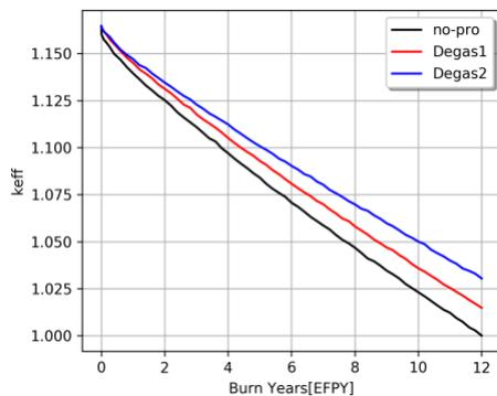
Figure 2. Deterioration of the effective multiplication factor with various depletion schemes
