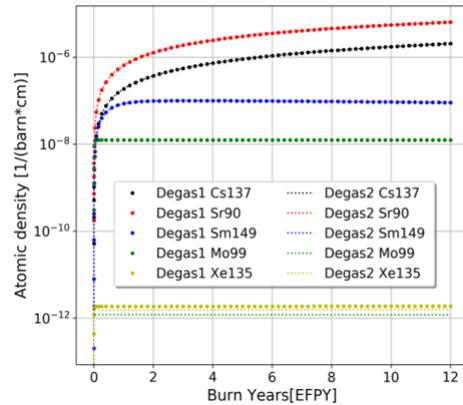
Figure 6. The atomic density of FPs in fuel salt of Degas1 and Degas2.
