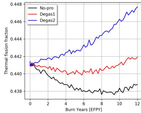
Figure 3. Development of the thermal fission fraction with various depletion schemes.
