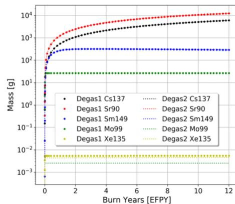
Figure 7. The mass of FPs in fuel salt of Degas1 and Degas2.
