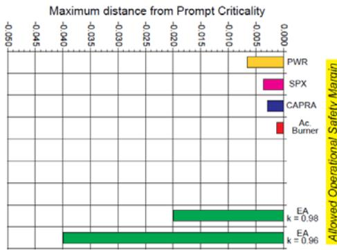
Fig. 3. Safety margin of a few types of nuclear reactors.
