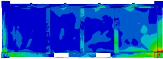
Fig. 5. Stress contour of the drop analysis at the third impact
