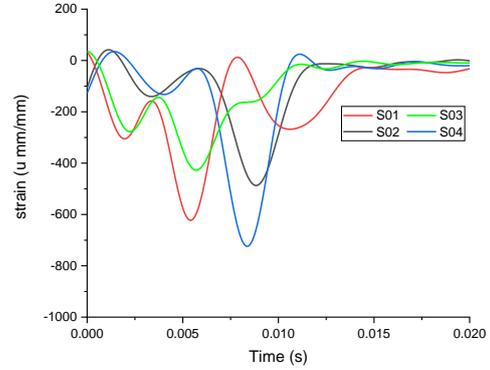
Fig. 2 Strain results of the drop test in the bottom drop (Cut-off frequency 300 Hz)
