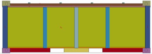
Fig. 3. FE model for the drop analysis of the IP-2 container
