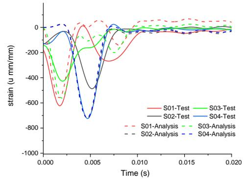
Fig. 6 Strain results of the drop test and analysis with the misaligned position
