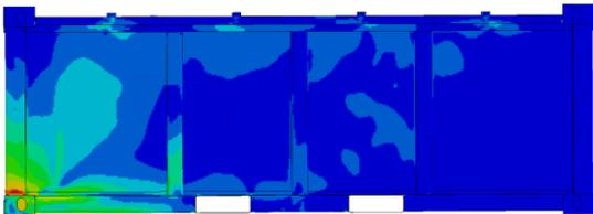
Fig. 4. Stress contour of the drop analysis at the first impact
