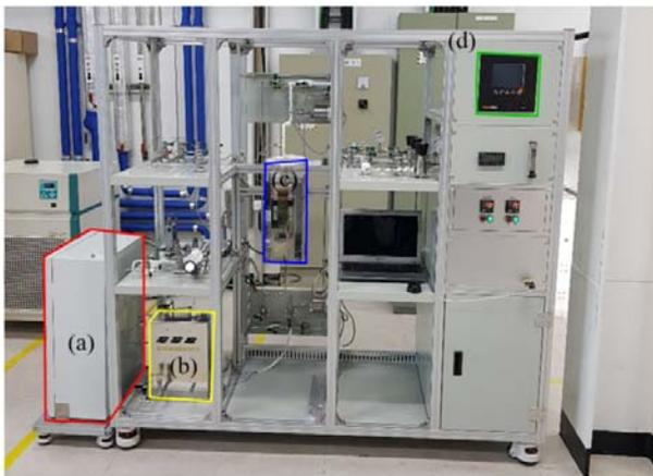
Fig. 1. Layout of AMSB apparatus ; (a) dryer, (b) vapor generator, (c) test section with furnace and (d) vapor analyzer
