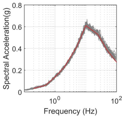
Fig. 3. Target spectrum and response spectrum by 30 sets of earthquakes.
