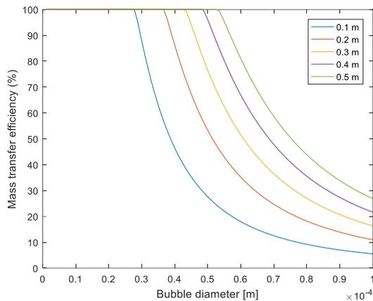
Fig. 7. Mass transfer efficiency as a function of bubble size
