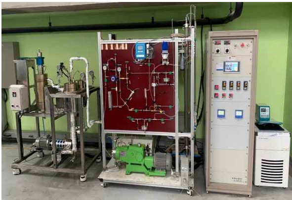
Fig. 5. Flow accelerated corrosion test facility at FNC Technology
