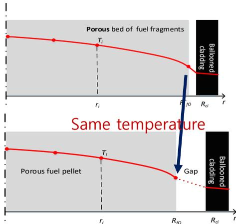
Fig. 1. Synchronized temperature distribution for crumbled fuel in ballooned clad
