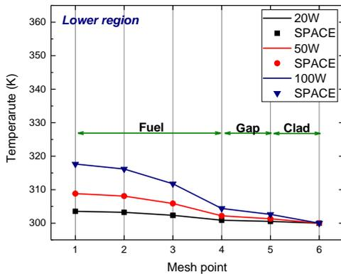
Fig. 5. Comparison of temperature radial distribution between calculated results and analytic solution at lower region ( $Z=0.3$  m)
