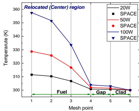
Fig. 4. Comparison of temperature radial distribution between calculated results and analytic solution at maximum ballooned region ( $Z=1.8$  m)
