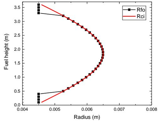
Fig. 2. Deformation pattern for conceptual problem (black line: fuel radius, red line: cladding inner radius)
