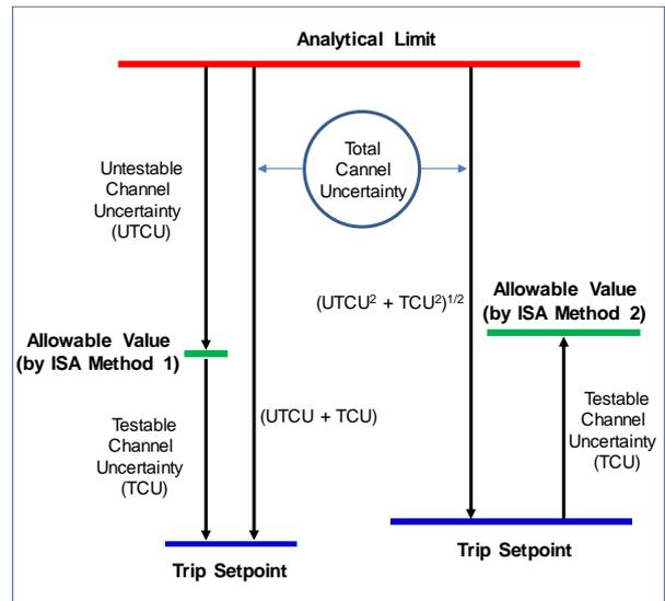
Fig. 1. ISA 67.04 allowable value calculation methods for rising trip parameter
