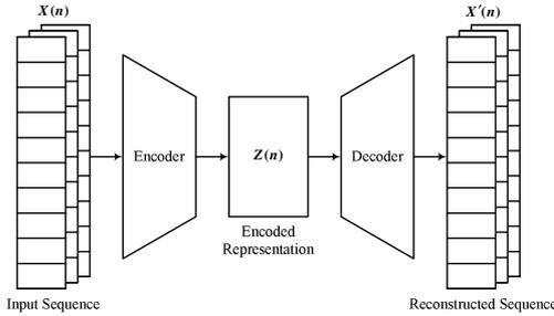
Fig. 2. LSTM-Autoencoder structure.
