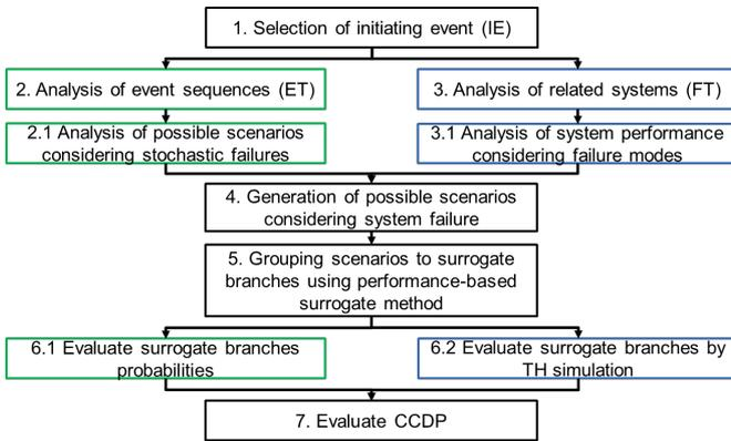
Fig. 1. The process of integrated dynamic PSA framework.
