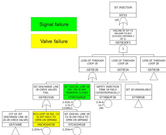
Fig. 4. Fault tree of SIT system considering possible failures.
