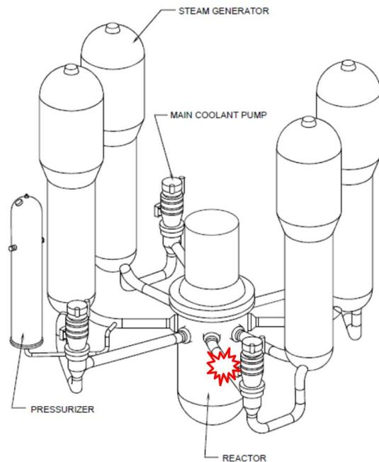
Fig. 2. Typical 4-loop PWR reactor coolant system configuration in LLOCA scenario.
