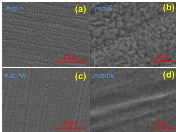
Fig. 2. SEM surface morphology of (a,b) PVD-Ti coatings on CS and (c,d) PVD-TiN coatings on CS.
