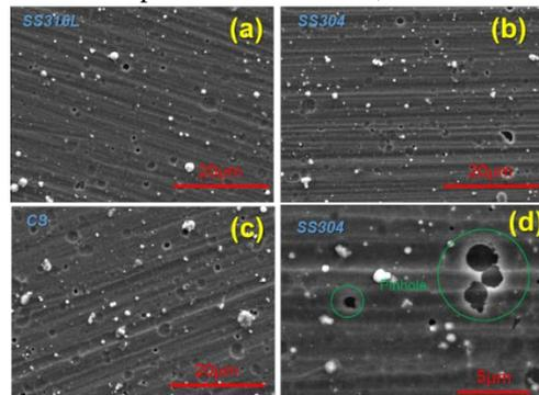
Fig. 1. SEM surface morphology of PVD-CrN coatings on (a) SUS316L, (b) SUS304, (c) CS, (d) SUS304-magnified.
