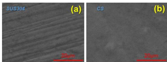
Fig. 3. SEM surface morphology of Ni electroless plating on (a) SUS304, (b) CS
