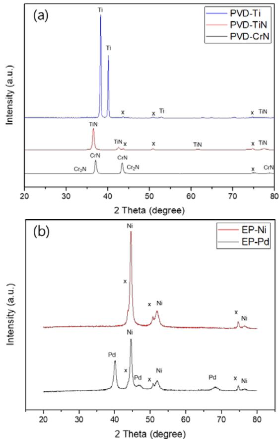
Fig. 6. XRD patterns of SUS304 specimens deposited by (a) PVD and (b) electroless plating.
