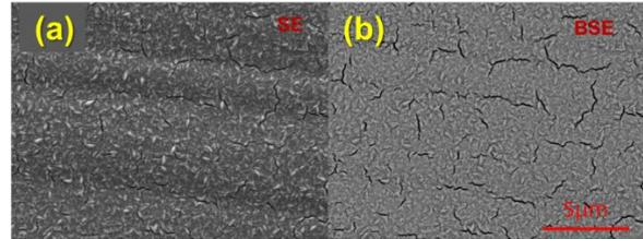
Fig. 4. SEM surface morphology of Pd electroless plating on SUS316L (a) SE mode, (b) BSE mode.
