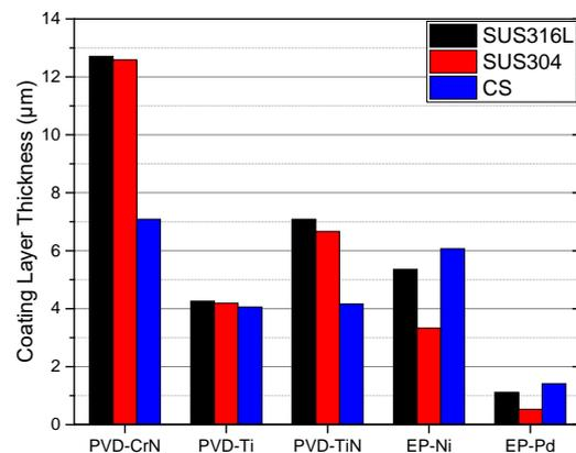
Fig. 5. The thickness of coating layer.
