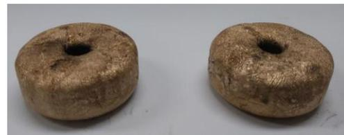
Fig. 7. Hollow cast billets with Cu-2.5wt%Si for extrusion
