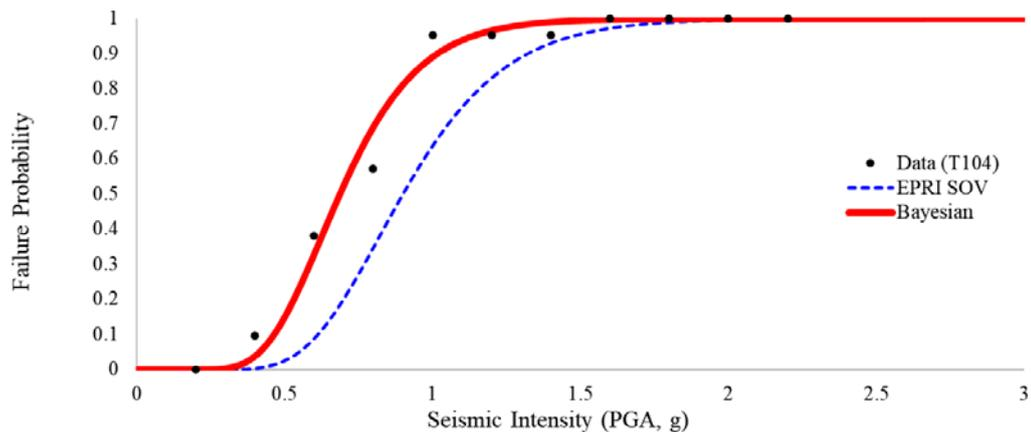
Fig. 3. Piping seismic fragility curves regarding T104
