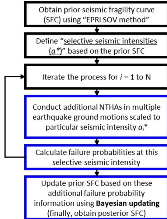
Fig. 1. Application of Bayesian updating to seismic fragility analysis
