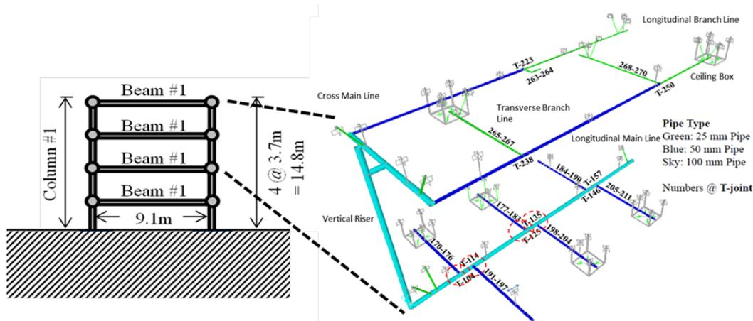
Fig. 2. Building-piping coupled numerical model
