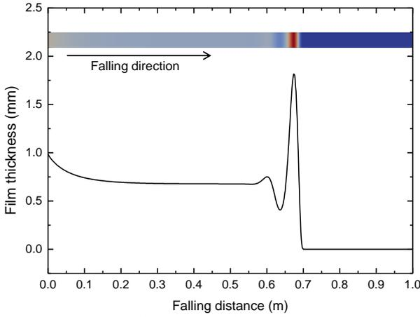
Fig. 1. Spatial distribution of the liquid film thickness at 0.5 seconds
