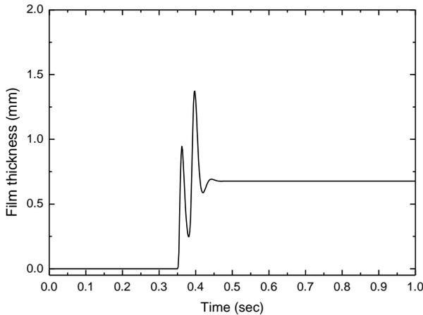
Fig. 2. Transient variation of the liquid film thickness at a height of 0.5m
