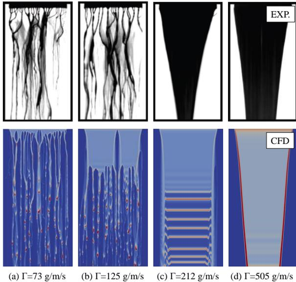
Fig. 3. Comparison between experiments and simulations for partially wetted film flow on a vertical plate
