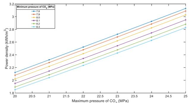
Figure 6. Power density vs Minimum pressure of system (Steam bypass fraction to HX of CCES: 0.5)
