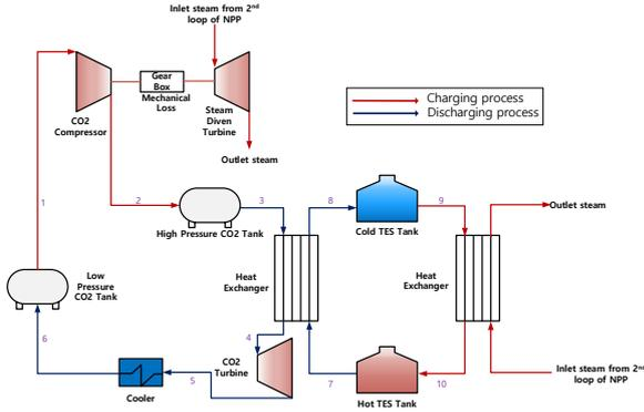
Figure 2. Layout of CCES integrated to PWR steam cycle
