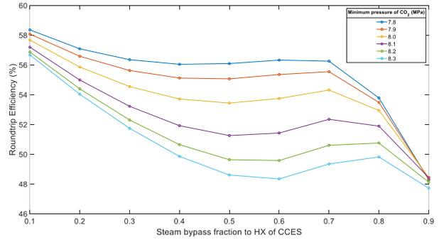
Figure 4. Round-trip efficiency vs Steam bypass fraction to HX of CCES (Maximum pressure of system: 25MPa)
