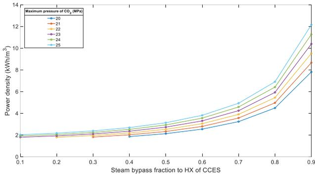
Figure 7. Power density vs Steam bypass fraction to HX of CCES
