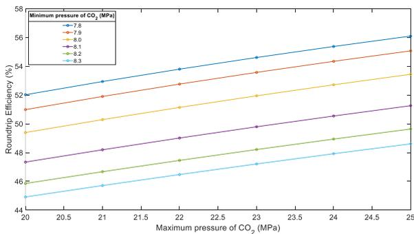
Figure 3. Round-trip efficiency vs Minimum pressure of system (Steam bypass fraction to HX of CCES: 0.5)
