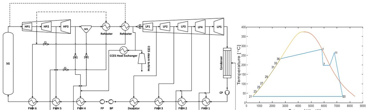
Figure 2. Layout and T-s diagram of Steam Cycle integrated with CCES
