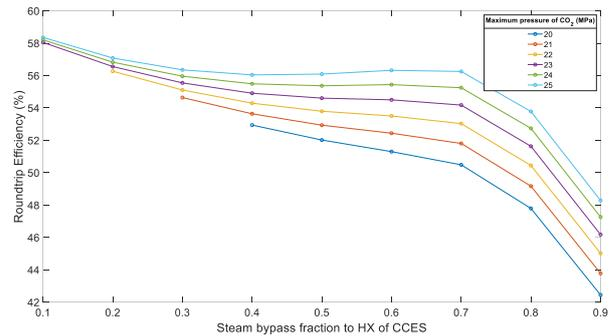
Figure 5. Round-trip efficiency vs Steam bypass fraction to HX of CCES (Minimum pressure of system: 7.8MPa)
