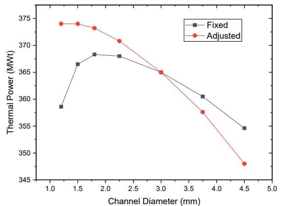
Fig. 2 Thermal power versus channel diameter
