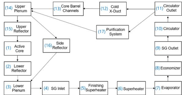
Fig. 2. POSCA model to simulate the primary circuit of the MHTGR-350.
