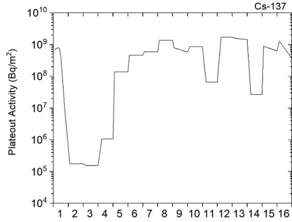
Fig. 6. 40-year plateout distribution of Cs-137 in the primary circuit of the MHTGR-350.
