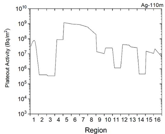
Fig. 7. 40-year plateout distribution of Ag-110m in the primary circuit of the MHTGR-350.
