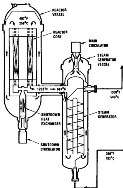
Fig. 1. Simplified flow diagram for the primary circuit of the MHTGR-350 [3].
