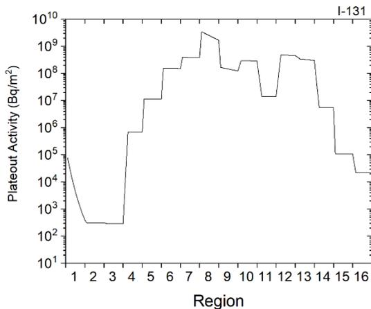
Fig. 5. 40-year plateout distribution of I-131 in the primary circuit of the MHTGR-350.
