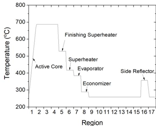
Fig. 3. Applied temperature distribution in the primary circuit of the MHTGR-350.
