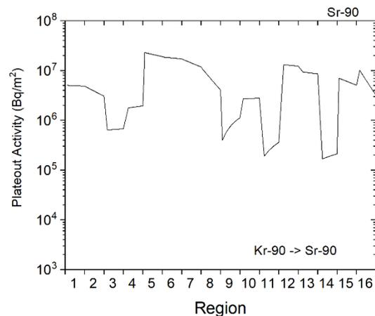
Fig. 8. 40-year plateout distribution of Sr-90 in the primary circuit of the MHTGR-350.
