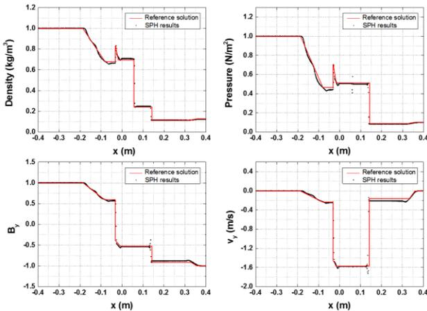
Fig. 2. Brio&Wu shock tube simulation results
