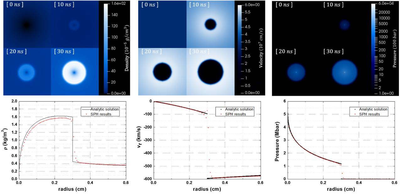
Fig. 5. Magnetized Noh Z-pinch simulation results from 2-dimensional SPH code
