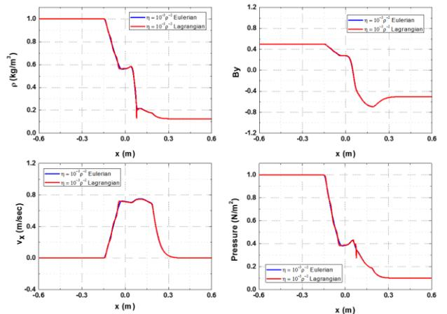
Fig. 4. Resistive MHD simulation results ( $\eta=10^{-3}\rho^{-2}$ )
