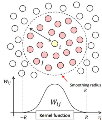
Fig. 1. Particle distribution with kernel function
