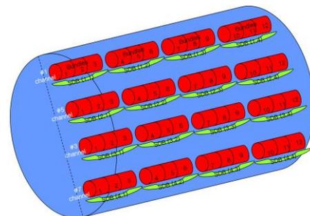
Figure 1 CANDU6 core nodalization (4x4) scheme in ISAAC
