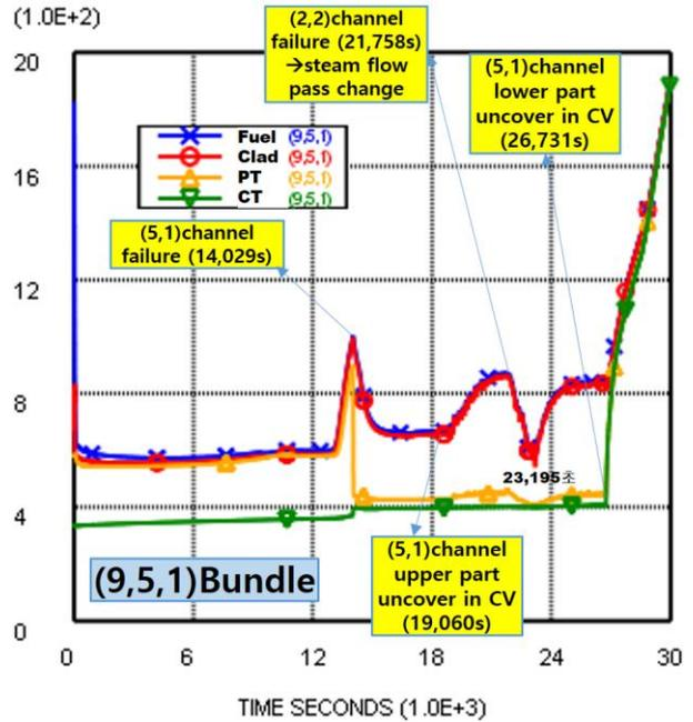
Figure 7 Lead Channel (= bundle(9,5,1)) Temp. Behavior
