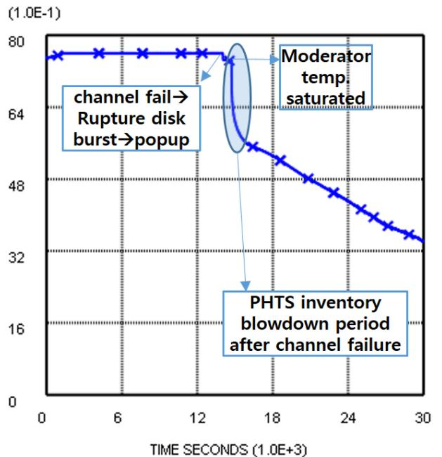
Figure 5 Moderator Water Level in CV
