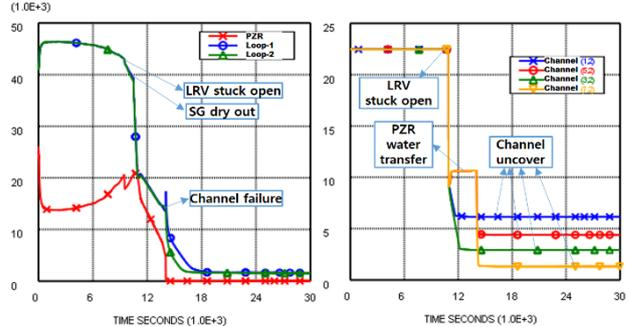
Figure 3 PHTS Water Inventory Figure 4 PHTS Water Level
