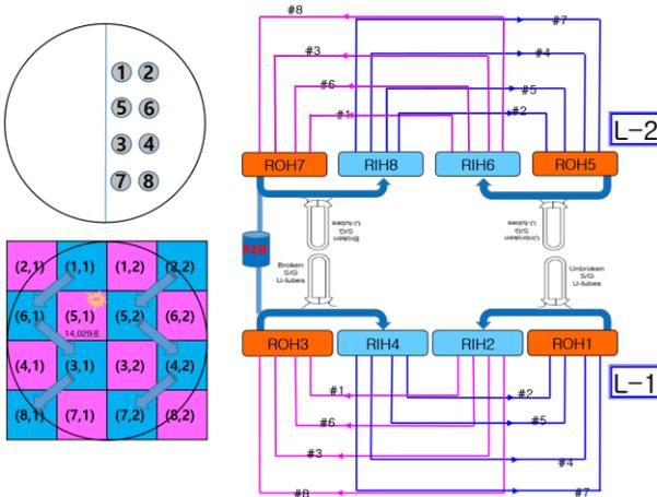
Figure 6 PHTS Core Passes (4x4) with Checker Board Pattern in ISAAC Modeling
