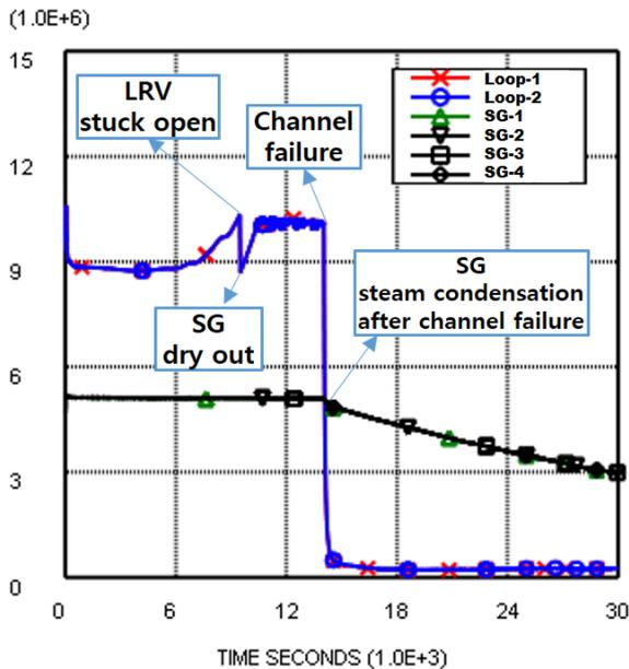
Figure 2 Pressure Behavior in the PHTS and SGs
