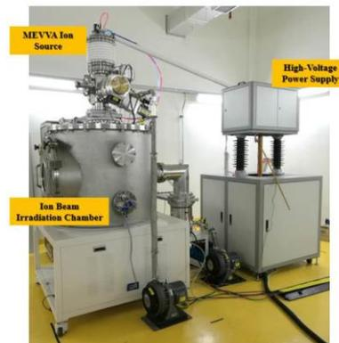
Fig. 1. The vertical ion beam facility and the MEVVA ion source.
