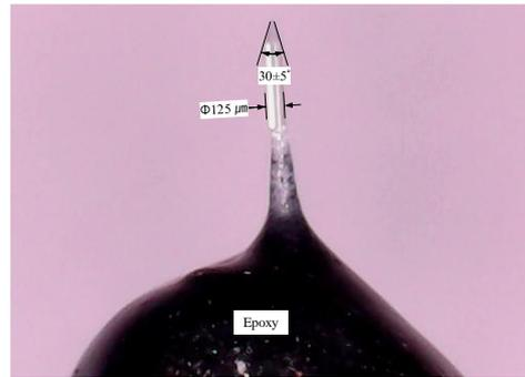
Fig. 2. The tip of OFP used for present experiment.
