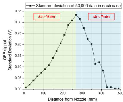
Fig. 4. Standard deviation of OFP signal by position.
