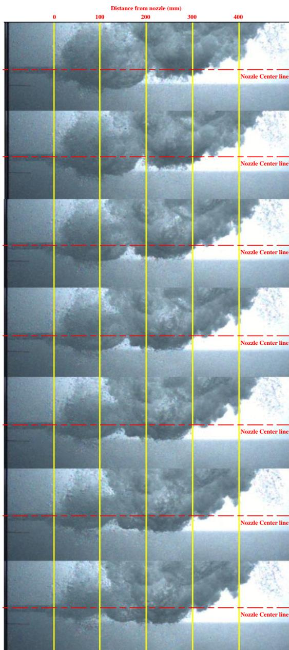
Fig. 5. The camera images of jet pool scrubbing
