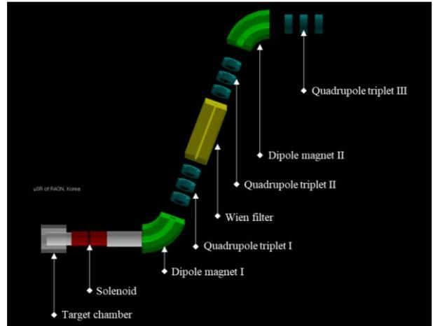
Fig. 1. 2D plot using G4beamline of muon beamline components at  $\mu$ SR facility.
