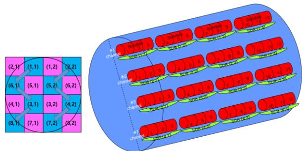
Figure 1 CANDU-6 core nodalization(4x4) scheme in ISAAC
