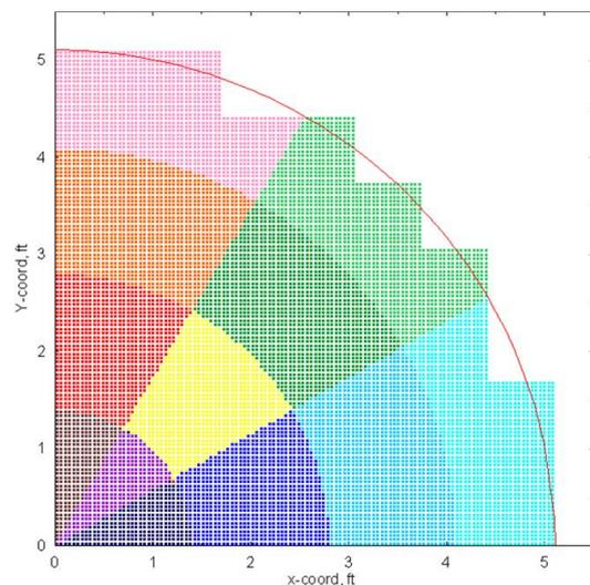
Fig. 2. Scheme of multi-dimension modeling of core
