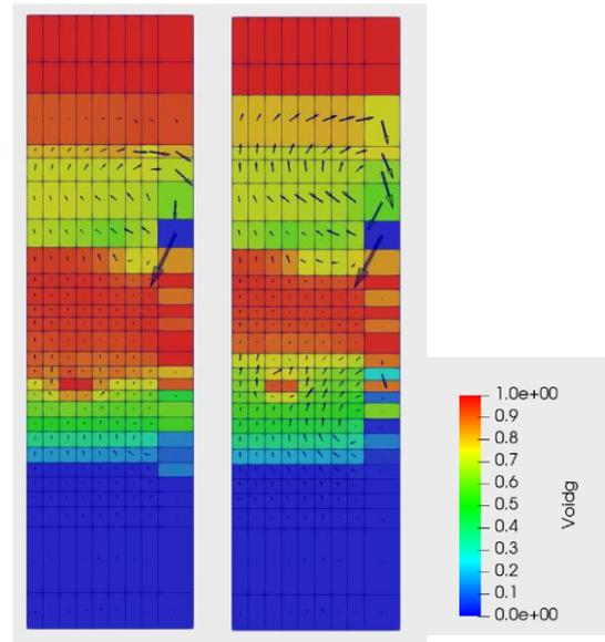
Fig. 1. Example of multi-dimensional flow pattern in a reflood test of SCTF.
