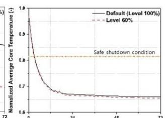
Figure 16. Avg. Core Temp., ECT level sensitivity
