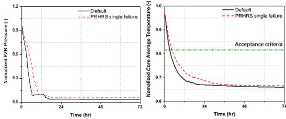
Figure 8. PZR pressure, PRHRS single failure
