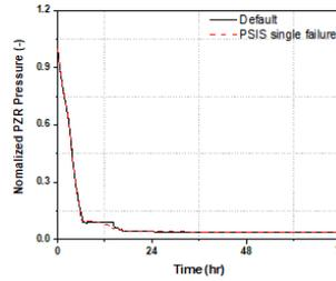
Figure 3. PZR pressure, PSIS single failure
