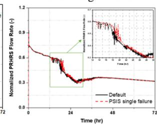
Figure 6. PRHRS Flow rate, PSIS single failure
