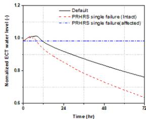
Figure 12. ECT water level, PRHRS single failure
