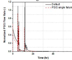
Figure 5. PSIS Flow rate, PSIS single failure
