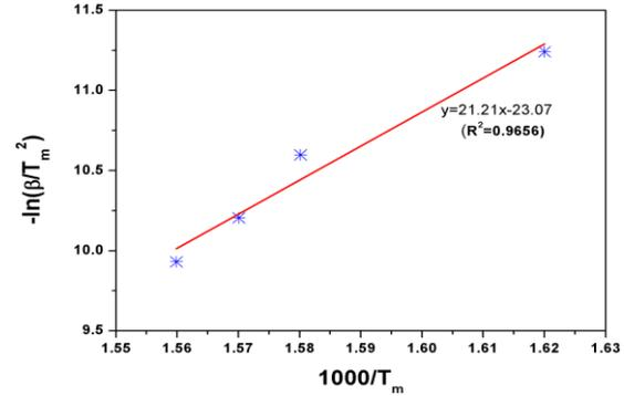
Fig. 2. Kissinger plot of cable samples.
