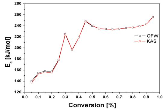
Fig. 3. Activation energies variation calculated via OFW and KAS method.
