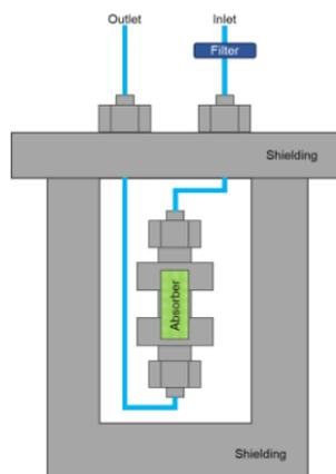
Fig. 1. Schematic diagram of  $^{82}\text{Sr}/^{82}\text{Rb}$  generator including inlet with filter, outlet, ion exchange absorber, and a thick shielding.
