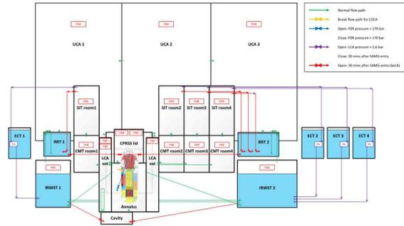
Fig. 1. Nodalization of SMART100 for MELCOR
