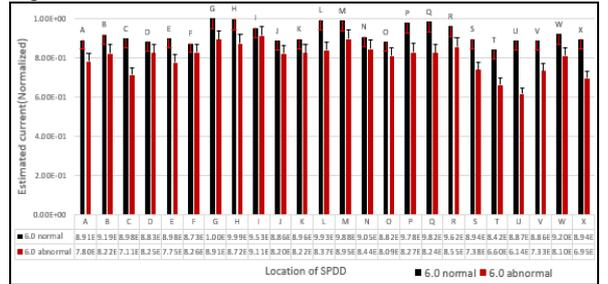
Fig. 10. Estimated current at each SPDD unit, 6.0wt% U-235
