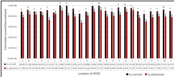
Fig. 7. Estimated current at each SPDD unit, 1yr cooled
