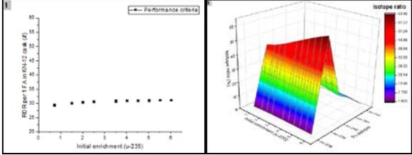
Fig. 3. RDR and Pu isotopes concentration with different initial enrichment
