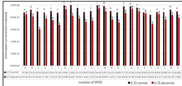
Fig. 9. Estimated current at each SPDD unit, 0.72wt% U-235
