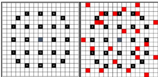
Fig. 4. Left : WH17x17 FA, Right : An example of test scenario with 23 dummy rods(RDR for 72GWD/MTU)
