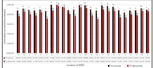
Fig. 6. Estimated current at each SPDD unit, 72GWD/MTU
