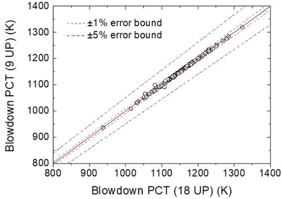
Fig. 2. Comparison of blowdown PCT from the regression analysis
