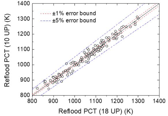
Fig. 4. Comparison of reflood PCT from the regression analysis
