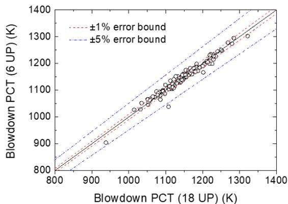
Fig. 1. Comparison of blowdown PCT from the correlation analysis
