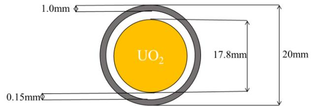
Fig. 1. Schematic cross-section image of a fuel rod
