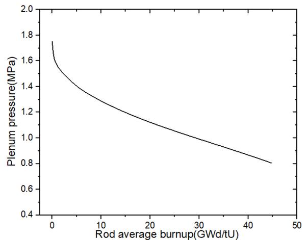
Fig. 5. Plenum pressure evolution
