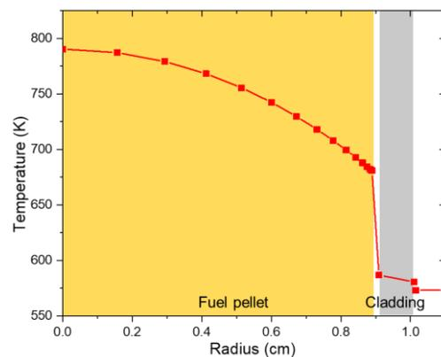
Fig. 2. Radial temperature calculation results at BOL
