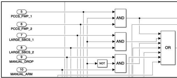
Fig. 3. Current RPCS inputs and partial logic circuit.
